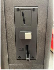
9. Pull the coin acceptor front and wiggle it loose. If this does not loosen the coin acceptor, pull off the top and push the coin acceptor out from within with your hand.
