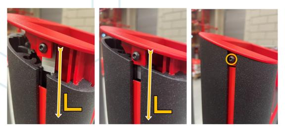
15. Screw it down until it is just tightened with the H2 Allan key.
