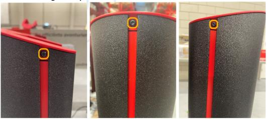
1. Unscrew the Inbus / Hex / Allan H2 screws. Note! Half a turn should be enough. In this way the iron tab won't loosen and fall in the pillar.
