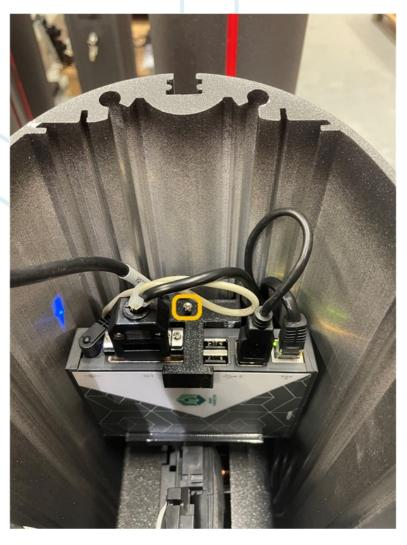
7. Unscrew the upper screw from the bracket. This bracket holds the SmartConnector in place. The bracket can be moved from the pillar. Disconnect the cable from the SmartConnector so it can be removed.
