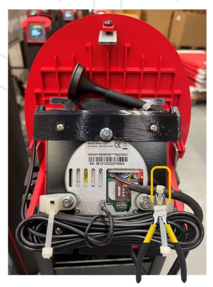
5. The connector will be locked in the Nayax module, but can be opened with a Phillips screwdriver by pressing the lock mechanism. The connector can be removed in this way.
