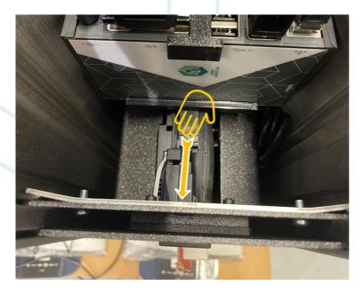
10. The coin acceptor is now dislodged and it can now be cleaned. Should the coin acceptor be replaced the top of the pillar and the SmartConnected should be removed, then remove the power of the coin acceptor.
